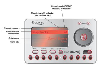
Figure 2. SKYFi Receiver display screen.
